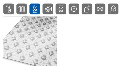
Deep-drawn pipe holding burls for stable fastening of KELOX multilayer pipes d16, connection of individual panels by overlapping. One long edge and one wide one as a reduced-size parent burl, marked with the KELIT logo between the parent burls; by preference, you should start installing on the right-hand side of the room. As a replacement for a clamping rail, PE screentone and fixing hooks
