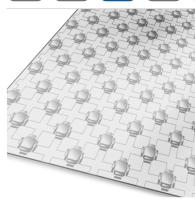
Deep-drawn pipe holding burls for stable fastening of KELOX multilayer pipes d16, connection of individual panels by overlapping. One long edge and one wide one as a reduced-size parent burl, marked with the KELIT logo between the parent burls; by preference, you should start installing on the right-hand side of the room. As a replacement for a clamping rail, PE screentone and fixing hooks
